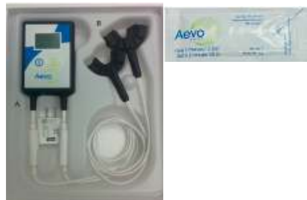
Gambar 1 LIPUS (Sistem Aevo) A elektronik genggam, B corong, dan C gel penghubung ultrasound. (Sumber: Kaur H, Bialy TE. Shortening of overall orthodontic treatment duration with LIPUS. J Clin Med 2020)
